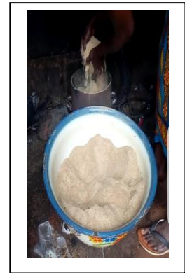
Figure 6. First 3kg rice husk being poured and compressed in the combustion chamber
